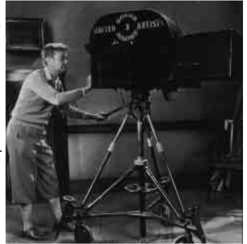
Struss in 1928 filming Mark Pickford in COQUETTE , her first sound film. Note the large "blimp" over the camera.
